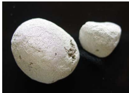
Two small clumps of mercury amalgam recovered from the wreck of the Atocha in 1984. They have a granulated texture and are quite soft.
